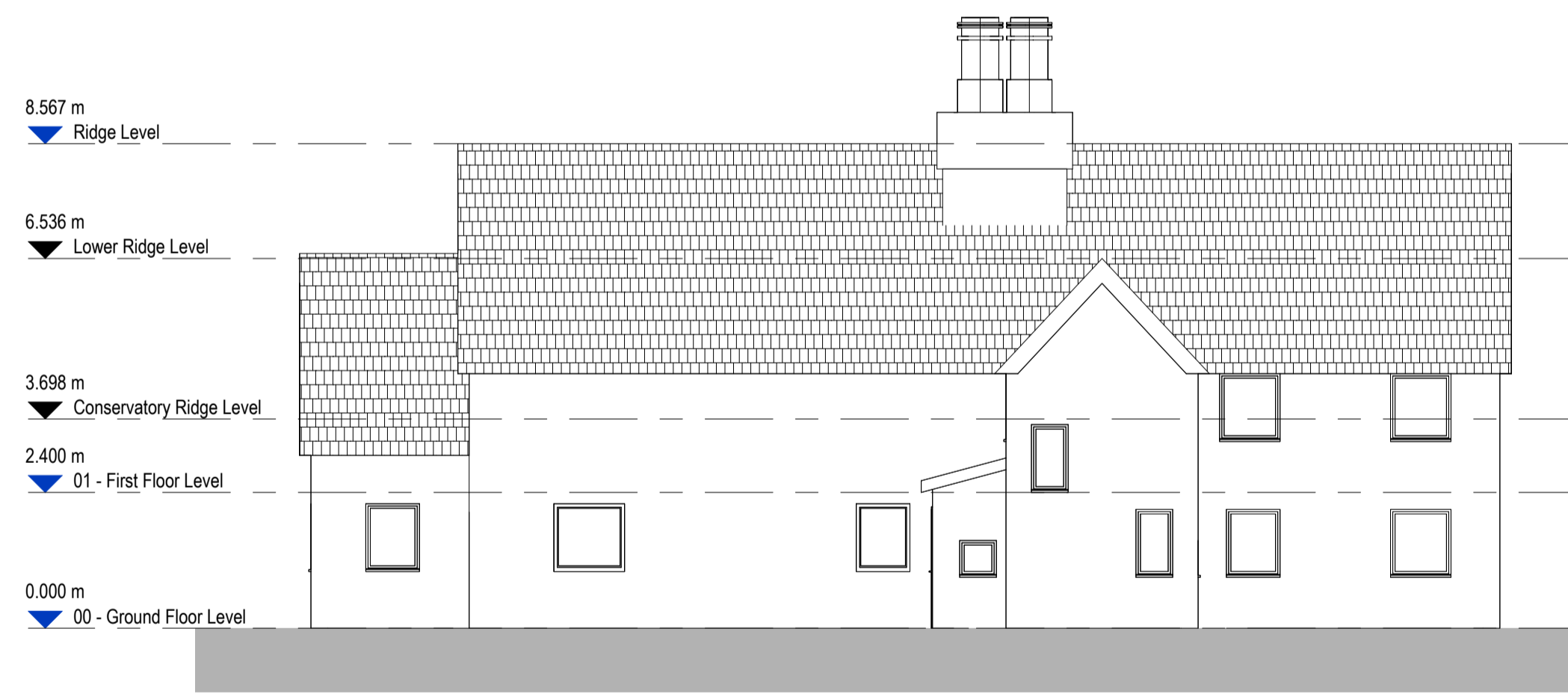
3 | 1 : 100 - Existing Elevation - South
